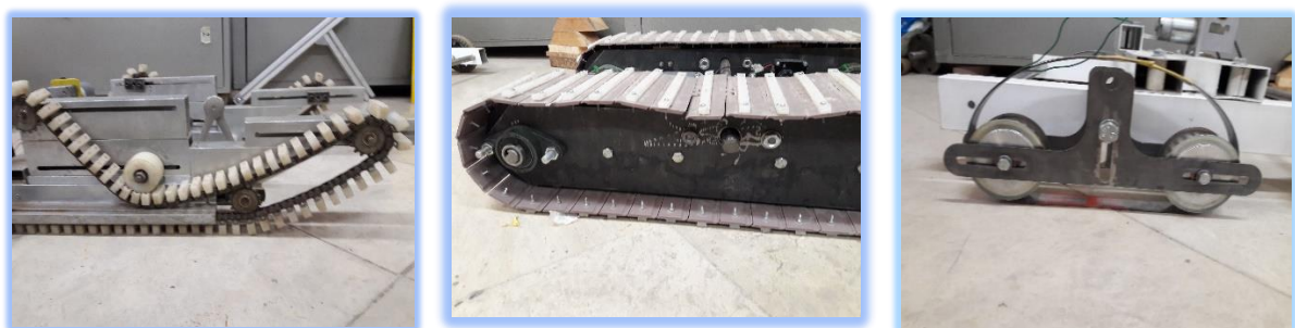
Figure 2. The tracked systems from right to left: flexible tracked, hinged tracked, four-bar tracked robots
