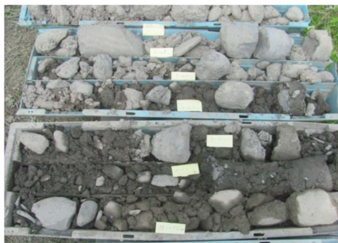
Photo 1. Sample of soil taken from the foundation of the dam.
